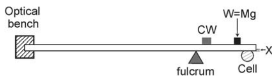
Fig. 7 A simplified schematic diagram of the pressure transducer setup. CW is a counterweight to balance the different torques of the two arms of the lever system (arm ratio \sim 4.2:1 ), W is the added weight, X is the deflection of the surface of the cell below the edge of a thin steel wedge at the short end of the lever arm and the optical bench is the same as that used for the volume flow measurements. Based on Fig. 2 of Barry (1970a)
